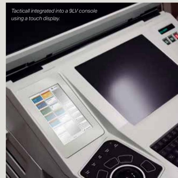
*TactiCall integrated into a 9LV console using a touch display.*
